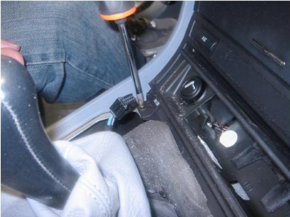
Use a plastic dash trim tool to carefully release the clips on the storage bin below the HVAC controls. You want to use caution on this step as you can damage the dashboard if you use too much pressure. Usually, once one side is free, the storage bin can be removed.
