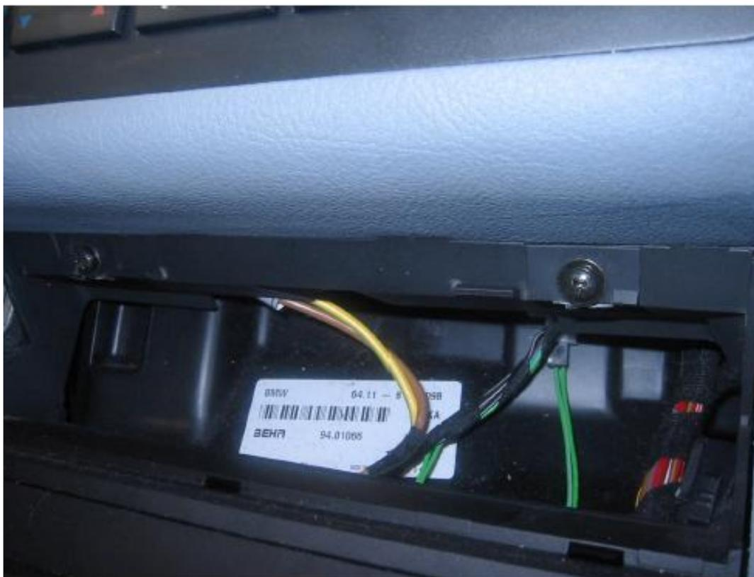
You will now be able to remove the ashtray carrier by pulling toward the back of the vehicle while at the same time, lifting up on the back of the piece to clear the shifter.
