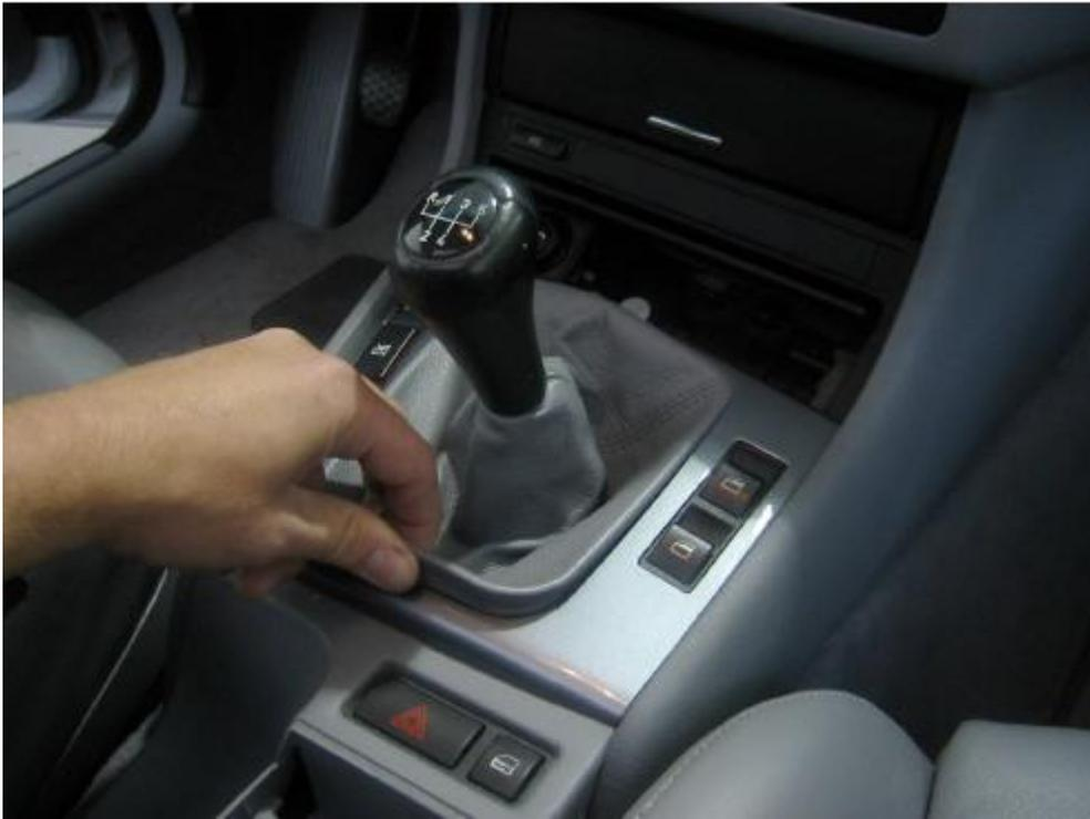
With the shift boot removed, you will see two Phillips-head screws. Remove the screws to allow you to remove the shifter surround.
