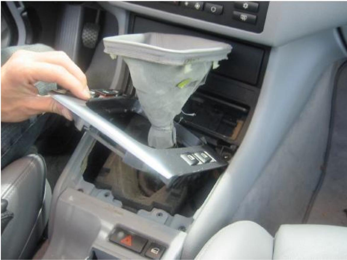
The connectors are unplugged by squeezing the locks found on their sides and gently pulling to unplug them from the switch. With the connectors undocked, you will be able to remove the shifter trim.
