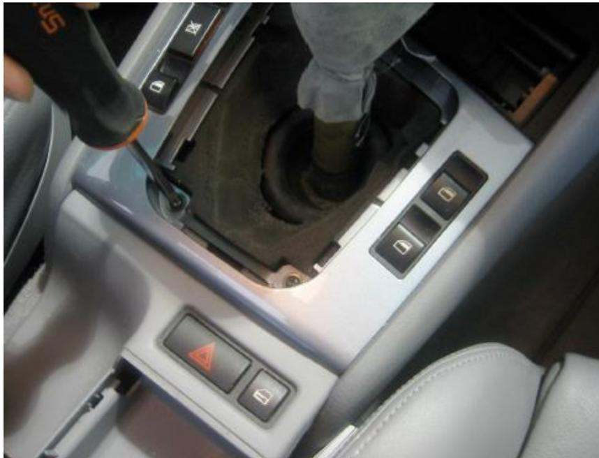
With the screws removed, you can lift up the rear edge of the shifter surround. Lift up and slide it toward the back of the car. You will need to flip the shifter surround up enough to unplug the power window connectors.
