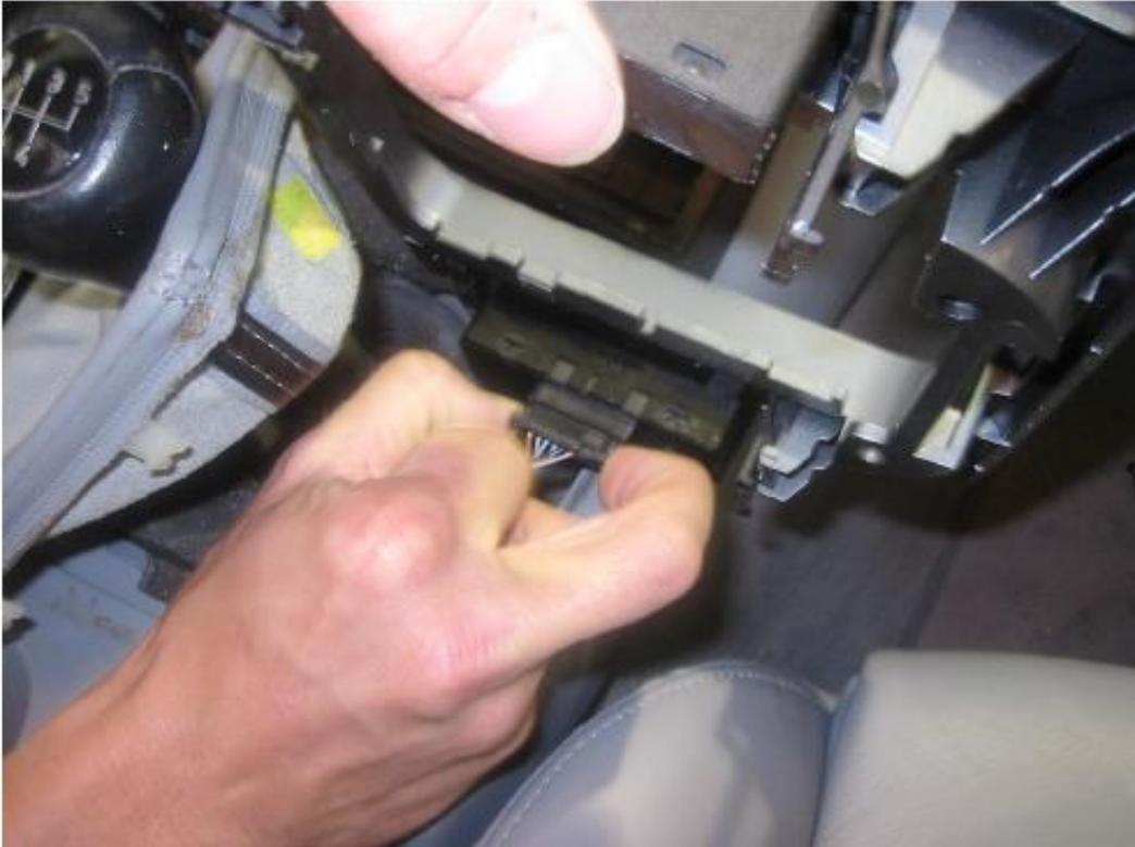
Remove the two more Philips-head screws located under the shifter surround.
