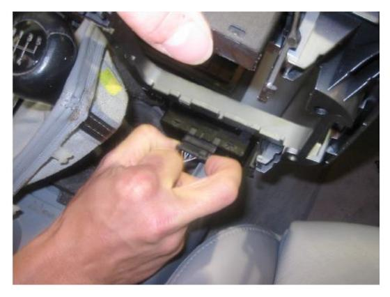
Remove the two more Philips-head screws located under the shifter surround.
