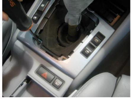
With the screws removed, you can lift up the rear edge of the shifter surround. Lift up and slide it toward the back of the car. You will need to flip the shifter surround up enough to unplug the power window connectors.
