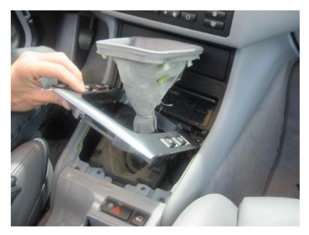
The connectors are unplugged by squeezing the locks found on their sides and gently pulling to unplug them from the switch. With the connectors undocked, you will be able to remove the shifter trim.
