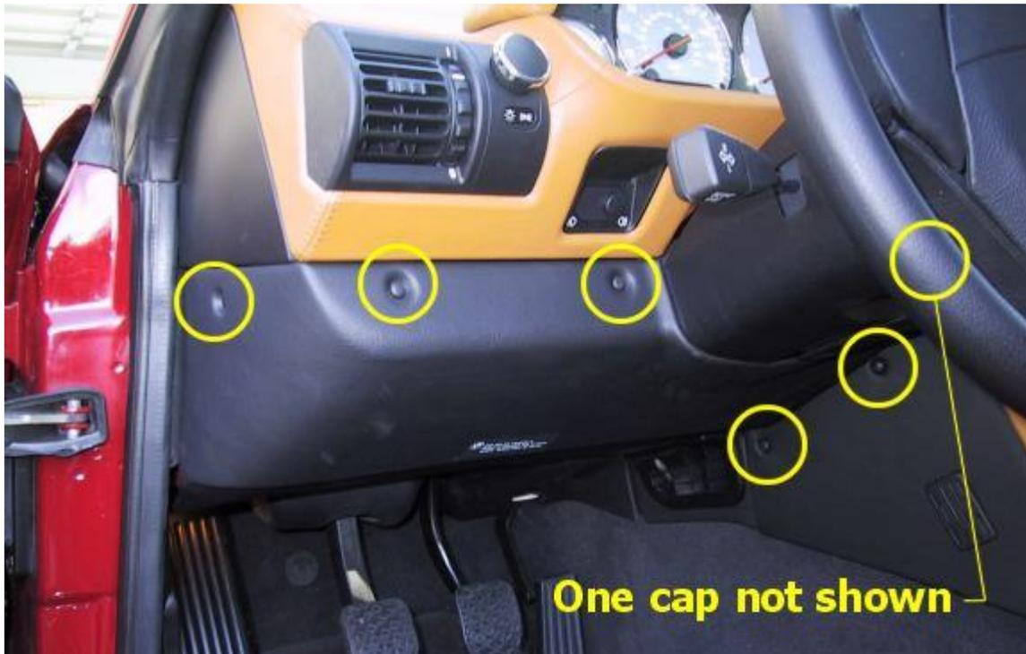
4. Remove the 6 screws underneath the screw caps. Pay attention to the types and locations of each screw. They are different sizes. We like to separate fasteners into envelopes while we work on cars. Write the location of each fastener on the outside of the envelope. This will make re-installation easier.
