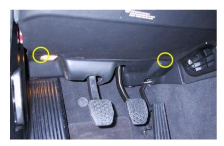
Once the fasteners are removed, you can remove the cowling entirely from the car. Pull it straight back towards the driver's seat.
