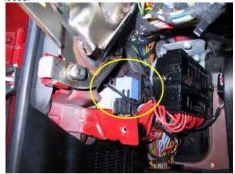
8. Install the DRL module. The text faces inboard and the locking tabs on the sides of the module point forward and aft in the car. Make sure it is fully docked and seated.
