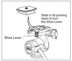
Keep the Shoe Lever unlocked, then sliding camera with the Quick Shoe in to the head, then automatically Shoe Lever is locking the Quick Shoe to hold. Please add locking tension by rotating Shoe Lever for sure, like double check.
