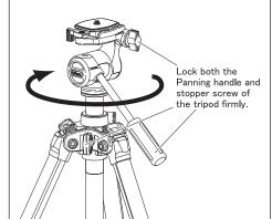
In order to connect to the tripod, lock all the screw on the head and tripod body firmly. Ensure the tripod screw attaching to the tripod, then rotate head toward Clockwise direction until it stops and locked
