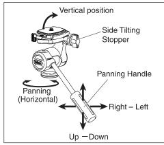
Release the Panning handle, and head turns to Up-Down also Right Left. Release Side Tilting Stopper, then camera plate turns to 90 degree for Vertical position. When the framing is decided, lock each stopper tightly for shooting.
