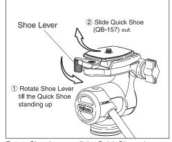
Rotate Shoe Lever until the Quick Shoe raises up automatically. Slide it out from the head then attach to the bottom of camera body. Then screw in carefully and tighten with a camera firmly.
