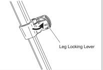
To adjust leg extension, raise up Leg Locking Lever and extend legs to the desired Position Then lock. Use upper part legs when it is not necessary to extend all legs till the maximum height.
