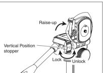
Unlock the Vertical Position Stopper, and turn camera plate to vertical position to 90° degrees for the portrait photo.
