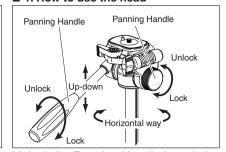
Unlock the Panning Handle by twisting to anti-clock wise direction, and can move up-and down. Unlock Panning stopper, and can move to horizontal way.
