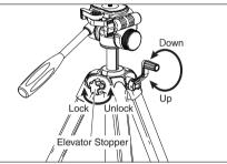
Unlock Elevator Stopper, and rotate Crank Handle to up or down to the desired height. Then lock the Elevator Stopper. (Hold your camera while operate the Elevator up or down.)
