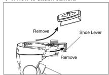
Raise up Shoe Lever until lock is released. Slide out the Quick-release to remove.
