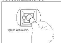
Adjust the screw to the bottom of camera body. Then tighten with a coin firmly.
