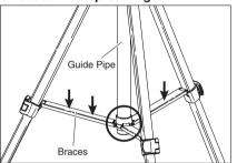
When spread leg angle, pull down the Guide Pipe till the end to spread braces tightly and steady. Make sure all legs come till the end to stand the tripod even.
