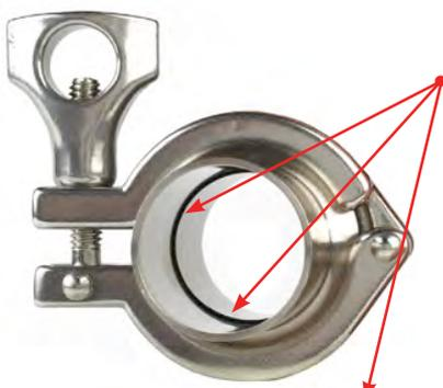
**Over torqued gaskets will pinch and extrude beyond I.D. of the sanitary ferrules and result in TOCs, bacterial buildup, and possible gasket tearing (see A below)**
