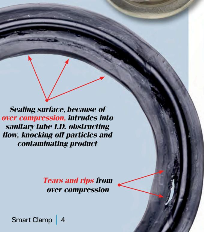
**Sealing surface, because of over compression, intrudes into sanitary tube I.D. obstructing flow, knocking off particles and contaminating product**
