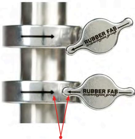
**Engaged Visual Indicator You know Smart Clamp™ is installed when the arrows are pointing to each other!**
