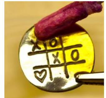
In some instances, there may be items or areas that you want to plate that you will not be able to attach the alligator clip to it. The item/area will not plate if it does not have the proper (-) electrical connection. In these situations a probe is used to make this connection in most of these circumstances. You will want to connect the alligator clip to the probe. Then use the probe to touch the surface area of the item being plated.
