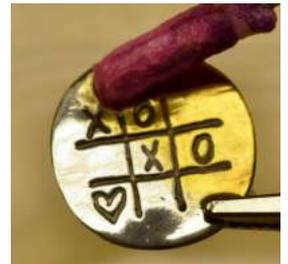
Note: If the area under the alligator clip is to be gold plated. You will need to reposition the clip in another spot during plating. A good technic is to move it about 3- 4 times in different locations on the item being plated during the plating process. This will allow a more even deposit of gold.
