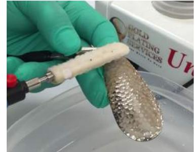
**\*Chrome Stripping Solution works the same as our electro-cleaner solution when in normal plating mode.**
