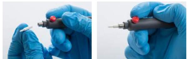
After the tip is inserted into the application handle the tip must soak in the pen plating gold solution until it is completely soaked through, normally 5-10 minutes for the first time used. Set the application handle into the Gold solution working beaker.
