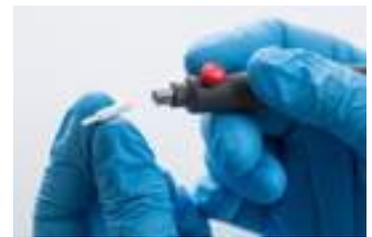
When you pull the application handle out of the working beaker for use, let the excess solution drip off back into the working beaker. There is a lot of gold in that solution – don't waste it!
