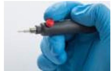
The fine tip will plate extremely high resolution such as the head of a quarter or a single finger on a printed circuit board as shown here. See picture to the Right.
