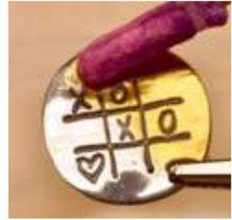
*Note: If the area under the alligator clip is to be gold plated. You will need to reposition the clip in another spot during plating. A good technic is to move it about 3- 4 times in different locations on the item being plated during the plating process. This will allow a more even deposit of gold.*
