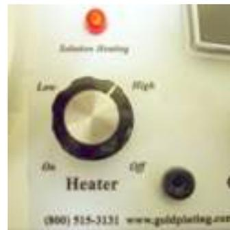
Because the *Perfect Temp* system is intended only to maintain proper solution temperature it will not quickly heat the solutions to operating temperature. **It can take up to 1 hour to raise the rhodium plating solution temperature from room temperature to 120° F.** Excessive solution warm-up periods can be avoided in several ways.
