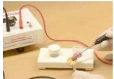
1. Plug the combination handle and red lead into the red (+) output port located on the right hand side of the machine underneath the plating voltage controller. Then plug the black common lead with an alligator clip into the black (-) output port located on the right hand side of the machine underneath the plating voltage controller.
