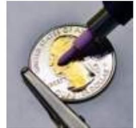
*Note: If the area under the probe is to be plated too; you will want to reposition it throughout the plating process.*
