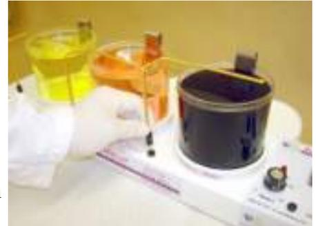
It is important to keep these buss bars clean so that electrical contact can be maintained between the buss bar and the rack. There may be times when you won't use the buss bars; you may want to simply hold the work in the common lead with the alligator clip. In this event, you can plug your common lead into any of the black (-) output ports on the front of the plating console.
