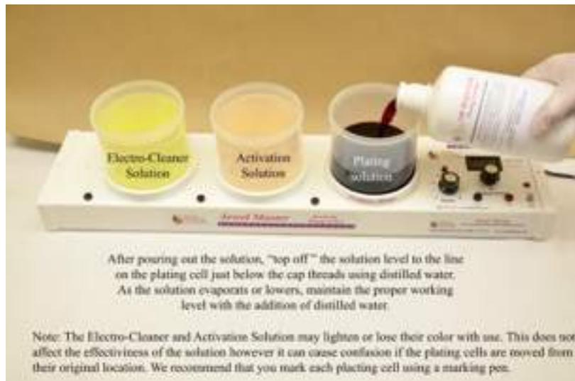
**\*When used, rhodium solution should be placed in the plating solution cell.**
