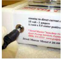
full range of output voltage should be between 0 VDC and 12 VDC when there is no plating load. All three plating cells will be controlled. Each solution will have its recommended voltage to use. We always suggest starting on the lower end of the recommended voltage and work your way up to meet your projects needs.
