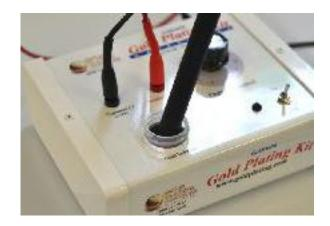
When you pull the application handle out of the working beaker for use, let the excess solution drip off back into the working beaker. There is a lot of gold in that solution – don't waste it!
