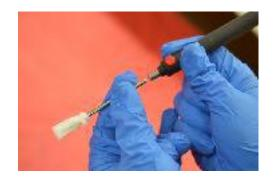
Install the bit into the application handle. Only about an inch of the bit will fit into the handle. Twist the red tightening screw snug; do not over tighten. Then place the end of the bit with the soaked sleeve into the working beaker with the solution.
