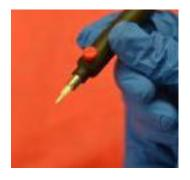
After the tip is inserted into the application handle the tip must soak in the 24k Gold Brush Plating Solution until it is completely soaked through, normally 5-10 minutes for the first time used. Set the application handle into the gold solution working beaker.
