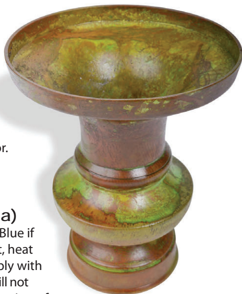
Above: Light Green applied to brass with plastic wrap.
