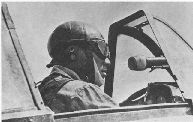
The telescope gun sight and flat canopy top identifies this as the early model of OSCAR. Japanese flying gear included a cotton hood that extended across the chin, worn under the leather helmet.
