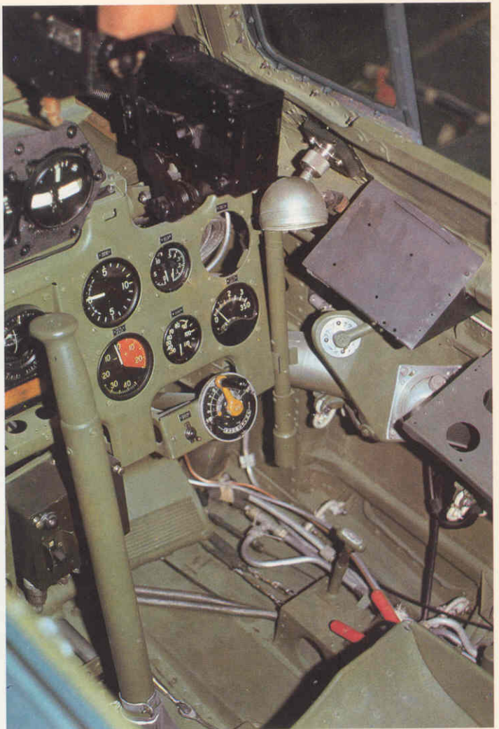
Above: Missing instrument should be a tachometer. Silver dome object is an adjustable cockpit light. Below: left side of cockpit showing engine controls. Mixture is forward red knob. Gun firing button is on the throttle handle.
