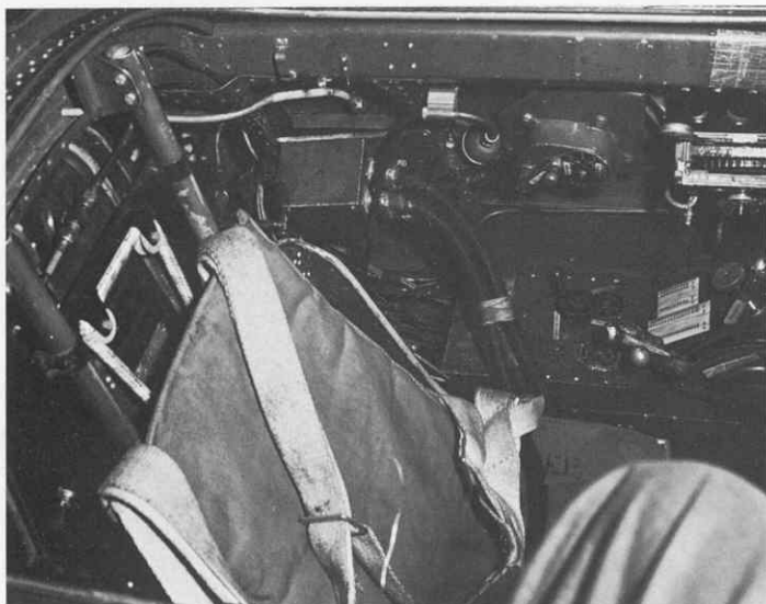
Left rear view of pilot's cockpit shows clearly that the entire area was painted interior olive green which is contrasted with black details.
