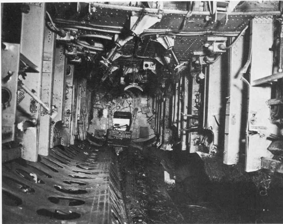
A wrecked HELEN found in New Guinea, May 1944, reveals full fuselage width bomb bay.
