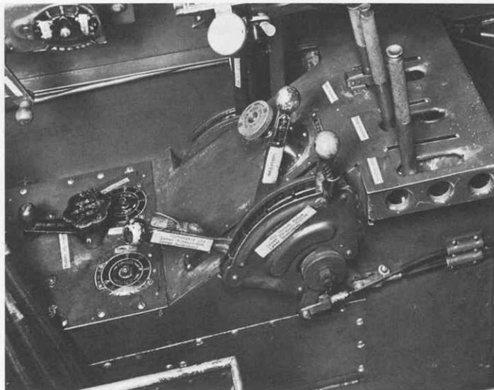
Pilot's left console with engine controls in center just below throttle knob at top of picture. Bomb and torpedo manual release handles are at the right in picture.
