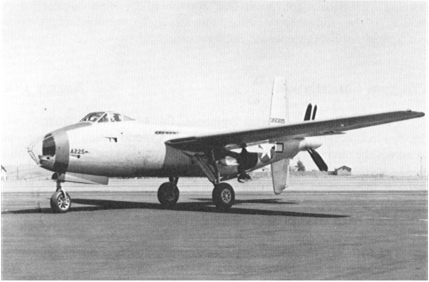
The XB-42 featured a novel engine-propeller arrangement.
