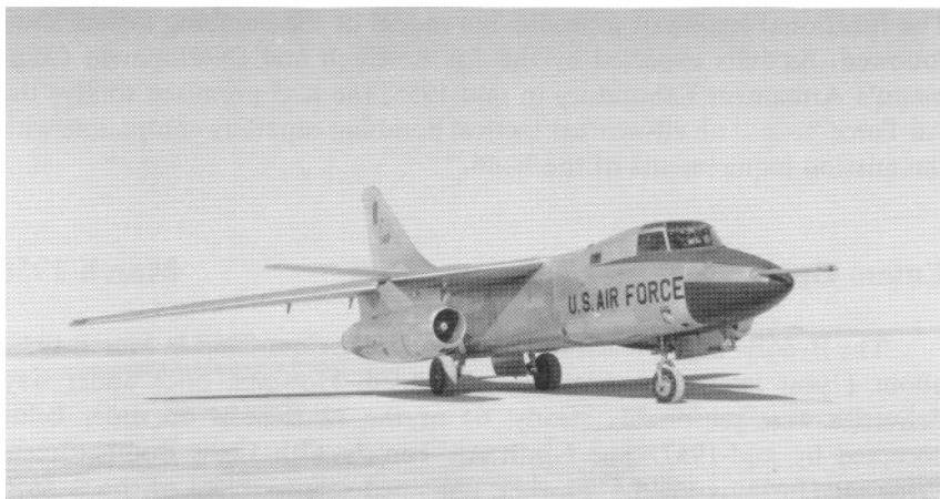
The B-66B featured the new K-5 bombing system and increased fuel capacity.
