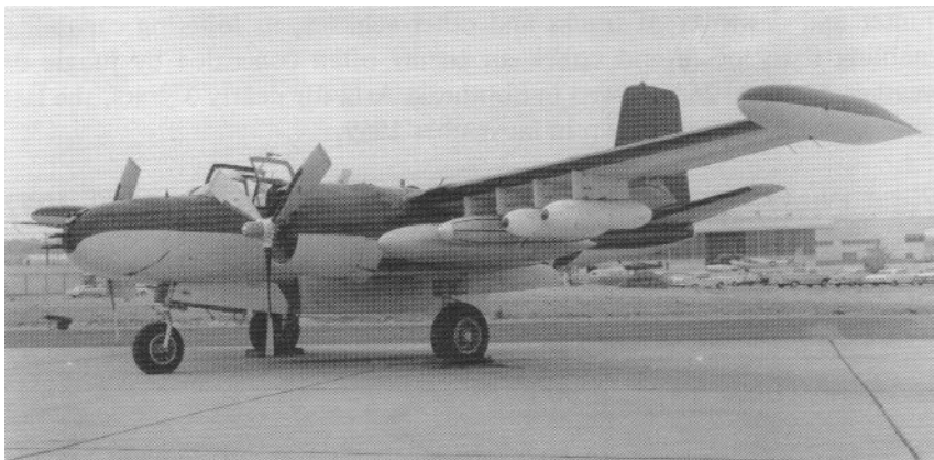
Specially modified for service in Vietnam, the B-26K featured permanent wing tip fuel tanks and various bomb and rocket pods.
