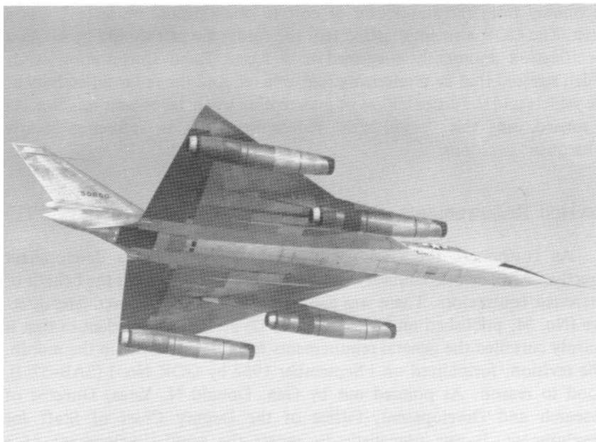
The delta-wing B-58 Hustler was powered by 4 General Electric J79 turbojet engines.
