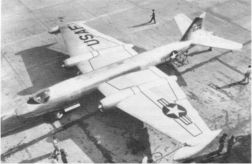
The B-57, an American version of the British Canberra, featured wing tip fuel tanks.
