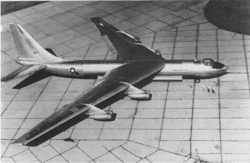
The prototype YB-60, a reconfigured B-36 with jet engines and swept-back wings.
