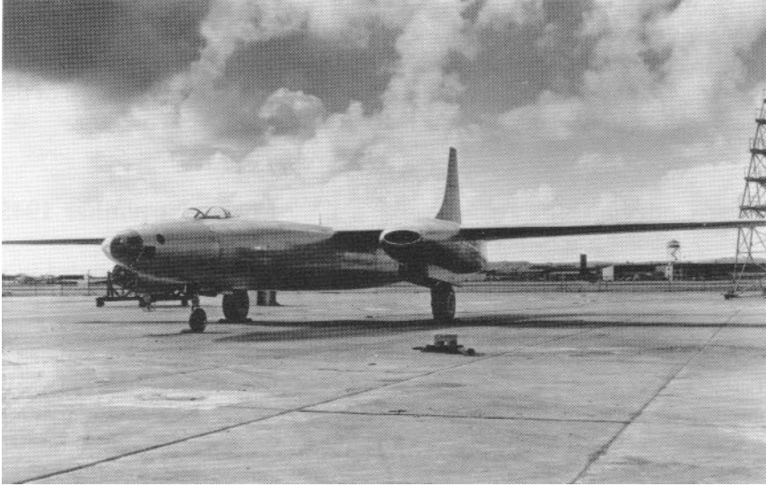
Long, thin wings and a teardrop canopy were special design characteristics of the XB-46.
