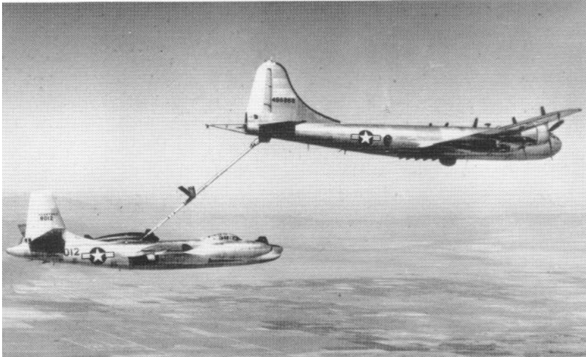
The RB-45C (left) was the first jet aircraft to be refueled in the air in this country. The tanker (right) is a KB-29A. 1950.
