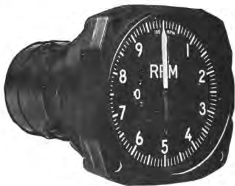
Figure 44.—Tachometer indicator dial.
