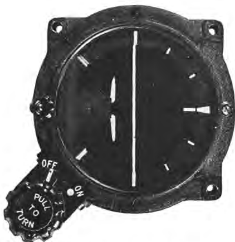
Figure 80.—Dial of a horizon indicator.
