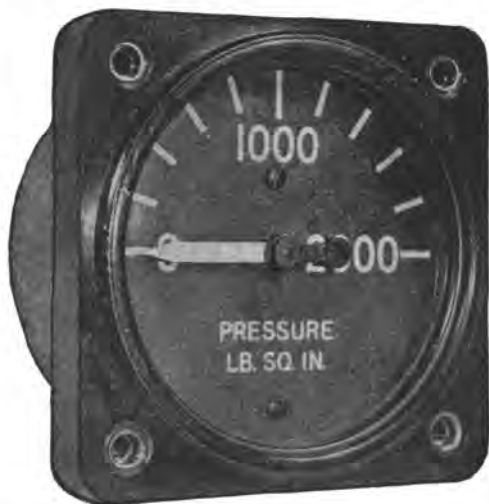
Figure 21.—Dial of a hydraulic pressure gage.
