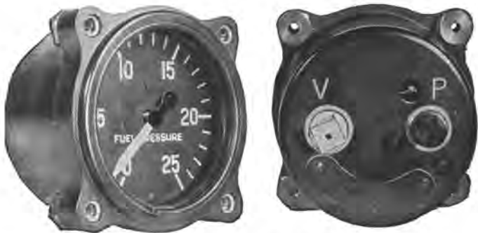
Figure 18.—Front and rear of fuel pressure gage.
