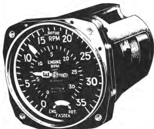
Figure 49.—Helicopter tachometer with synchroscope.
