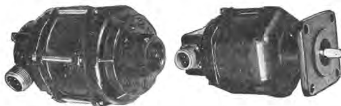
Figure 45.—Tachometer generators—right, stud type; left, screw type.
