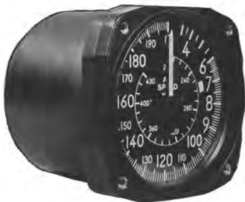
Figure 28.—Dial of 430-knot airspeed indicator.
