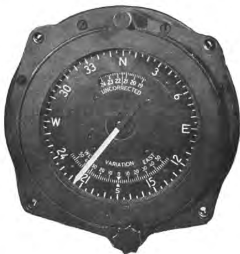
Figure 61.—Master indicator, gyro flux-gate compass.
