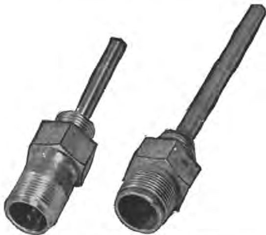
Figure 39.—Resistance thermometer bulb assemblies.
