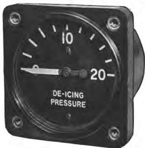
Figure 19.—Dial of a de-icing pressure gage.
