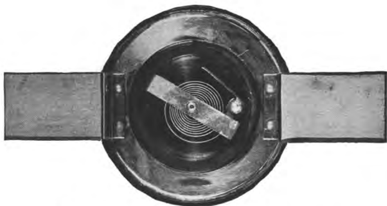
Figure 34.—Bi-metal spiral in outside air thermometer.
