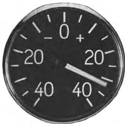
Figure 35.—Bi-metal thermometer dial.
