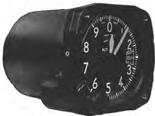
Figure 30.—Dial of a sensitive altimeter.
