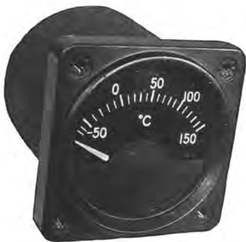
Figure 37.—Indicator of an electrical resistance thermometer.
