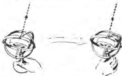
SUPPORT SWUNG IN ARC - GYRO AXIS CONTINUES TO POINT IN SAME DIRECTION
