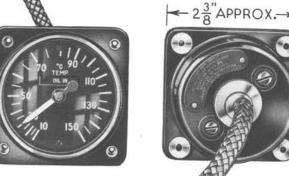
RELATIONSHIP OF PARTS: The bulb, capillary and indicator are permanently fitted together.
