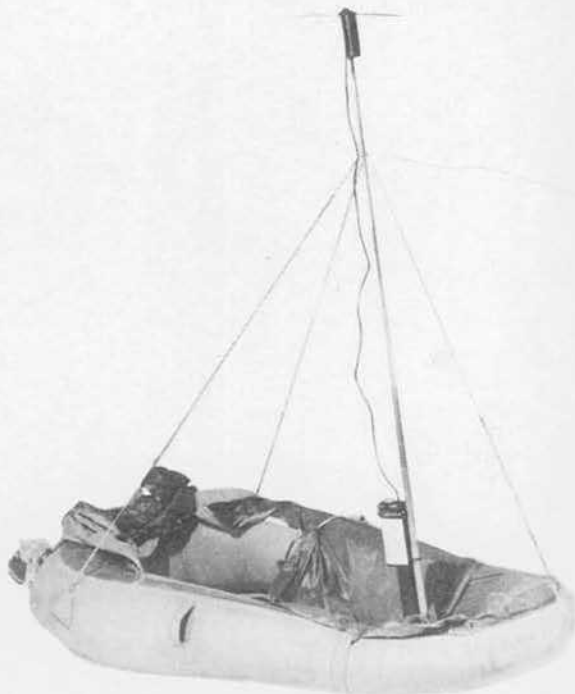
Radio Set AN/CPT-2 is installed in life raft after being forced down and operates automatically.
