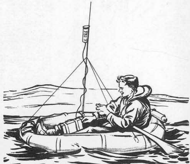
Sea Rescue Beacon Transmitter AN/CPN-16, 16X for use in one-man life rafts.
