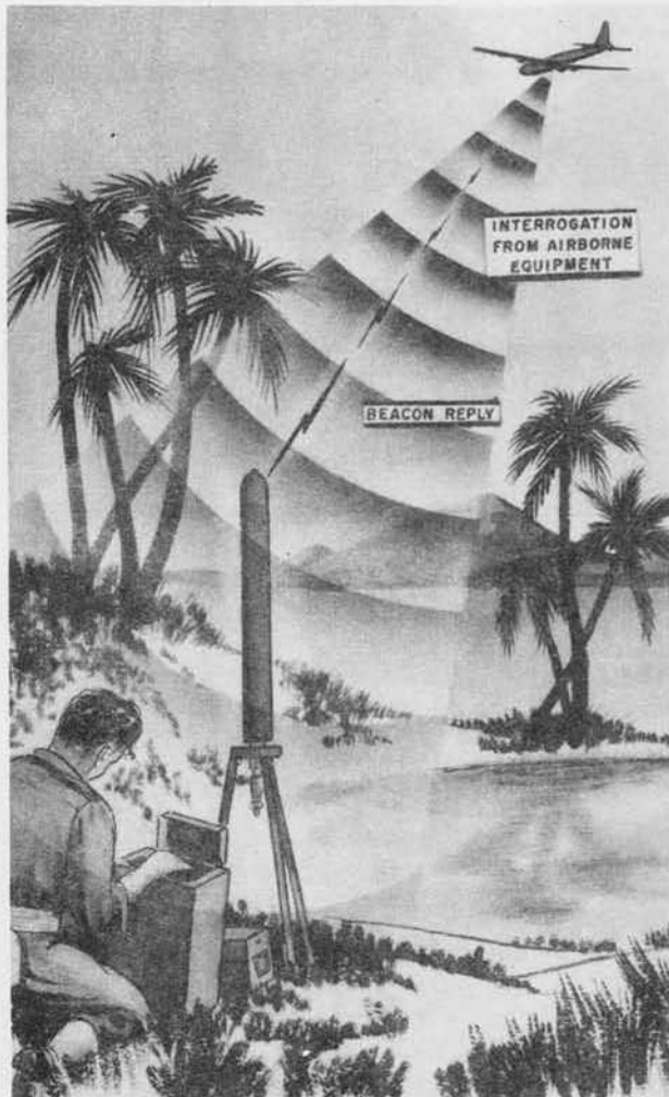
Aircraft Interrogation Triggers Beacon Reply which establishes its identity & position in range and azimuth.
