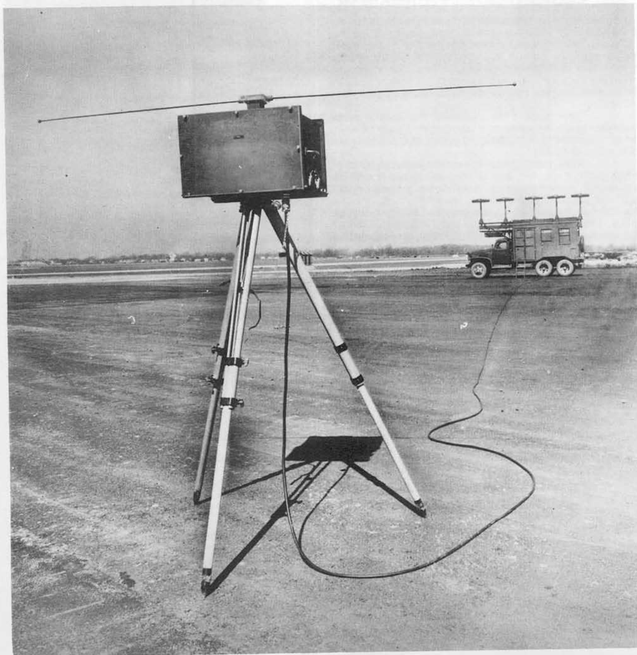
Course Detector BC-753 is generally placed well away from and parallel to antenna equipment RC-109.
