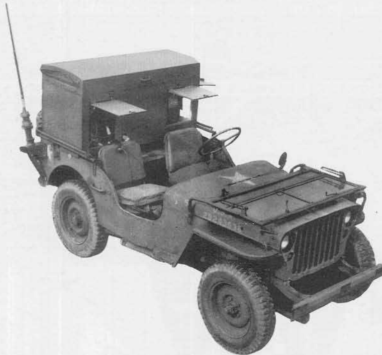
1. Radio Transmitter BC-902-B 2. Radio Set SCR-610-A 3. Power Unit PE-88 4. Shelter S-2/MRN-3 5. Roll BG-56
