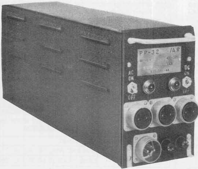
Rectifier Power Unit PP-32/AR
