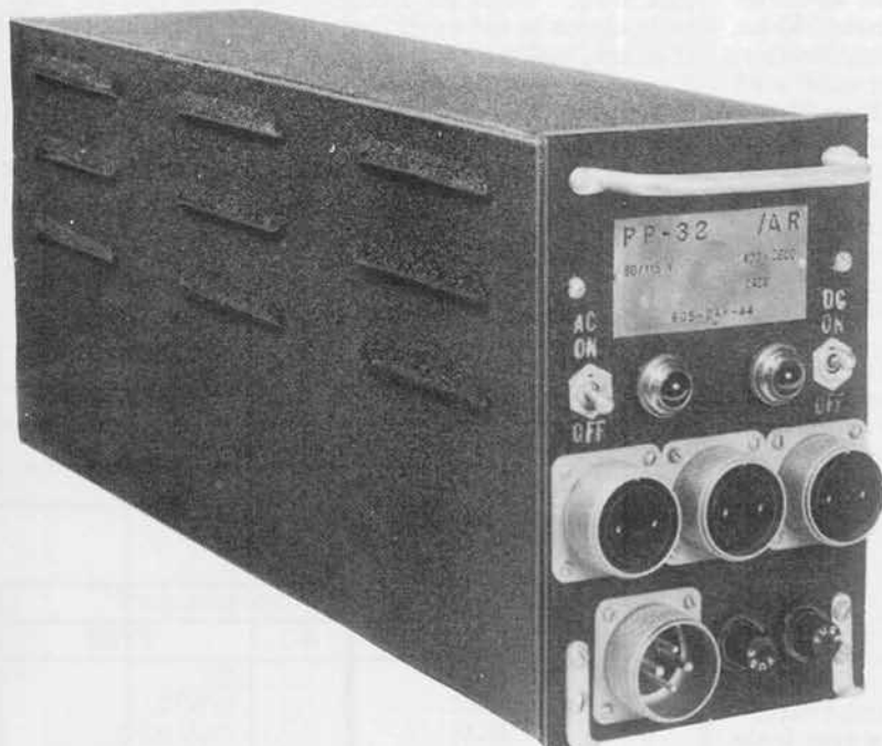
Rectifier Power Unit PP-32/AR
