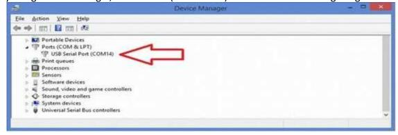
**22A. Set Up Procedure:** Allow the computer to assign a com port and install FTDI drivers manually, as needed. Device drivers are located in C, Program Files, International Light Technologies, Datalight III, FTDI folder. To install drivers double click driver CDM.....exe
