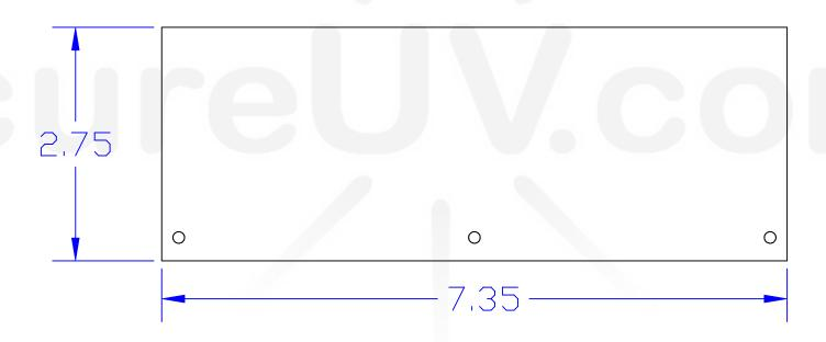
SET CONSISTS OF 2 PIECES ALL DIMENSIONS SHOWN IN FLAT MATERIAL THICKNESS 0.020"
