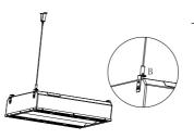
Step 2: Tighten hexagon screws shown in figure B
