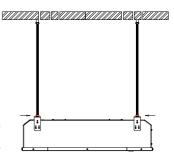
Step 3: Adjust the lamp and tighten the boom screw to fix it on the installation accessories (Remark: the threaded rod is M8)
