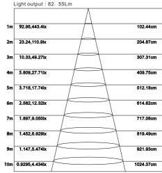
height Eavg,Emax Average beam:54.24angle diameter
