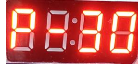
Figure 12: Waiting for user to press 30 minutes button on the remote control.
