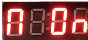
Figure 8: Safety motion detection enabled confirmation message.
