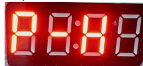
Figure 15: Waiting for user to press HOLD button on the remote control.
