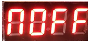
Figure 7: Safety motion detection disabled confirmation message.
