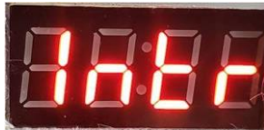
Figure 5: Unit interrupted by motion detection while the time-out counter is greater than zero.
