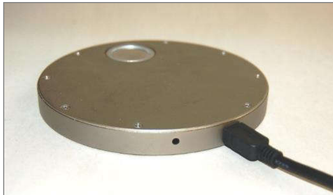
Connecting a Radiometer via the radiometer's mini-USB connector
