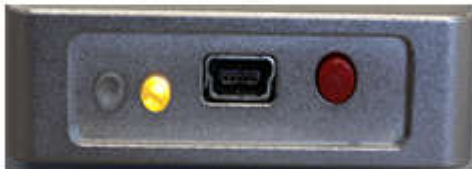
Flashing Yellow LED: Unit in Pause
