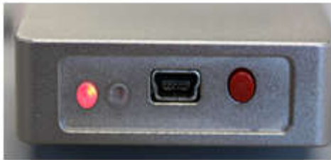
Flashing Red LED: Unit On and in Standby mode
