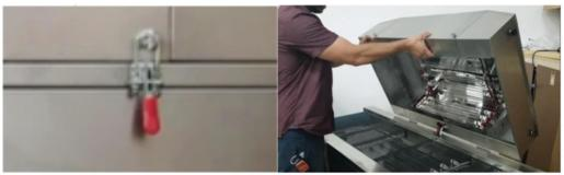
Once all the required bulbs are replaced, gently lower the top and redo the catches. It is recommended that if the unit is in heavy use, all bulbs are replaced every 12 to 18 months.
