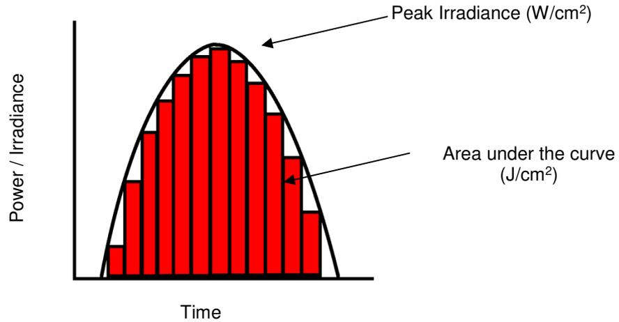
Energy Density is the total amount of energy exposure over time. It is the mathematical calculation of the area under the irradiance curve. The instrument calculates energy density by adding many irradiance samples together. The numerical irradiance reported is the peak irradiance value recorded by the instrument
