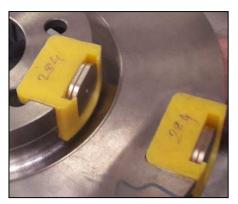
Left: Image showing the two MicroCure case halves with the printed circuit board 'sandwiched' between the two halves. The case halves are used to communicate with the EIT DataReader
