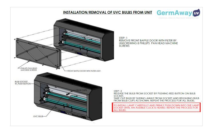
Step 1: Remove Front Door with Filter by unscrewing 8 captive screws.
