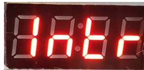
Figure 4: Unit interrupted by motion detection sensor while the time-out counter is greater than zero.
