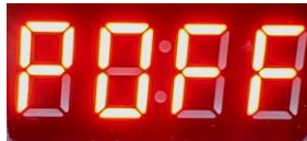
Figure 10: Waiting for user to press OFF button on the remote control.
