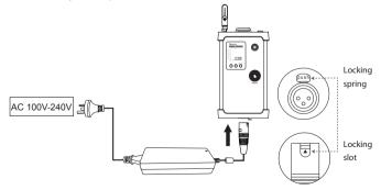
\* Please pull the power adapter out by pushing the locking spring down on the controller box.
