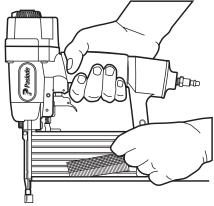
**Step No. 3** – Push the magazine firmly towards the front of the tool until it locks in place. The tool is now ready for use.
