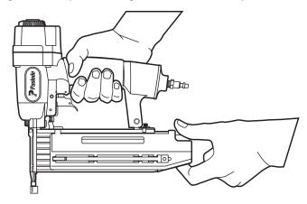
**Step No. 2** – Insert the strip of 18 gauge finish nails with the point of the fastener facing down and place the point of the fastener into the **bottom** of the magazine channel. Placing fasteners on the top of the magazine will cause jamming.
