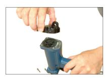
Release *Screws(501)* and take away *Cap(001)*, *Packing(002)* and *Bumper(003)*.
