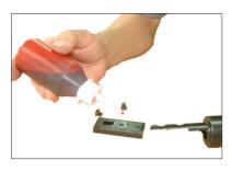
Reassemble New Driver Guide (016) and *Screws*(520).
