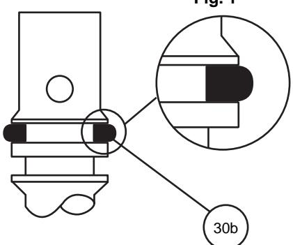
**Installation Note:** When installing three “D” seals (30b) on trigger valve stem, insure seals are seated properly and not twisted (see figure 1 for proper installation).
