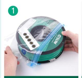
Put 3D filament, Humidity Indicator and Desiccant in the bag.
