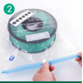
Seal the vacuum bag with Sealing Clip.
