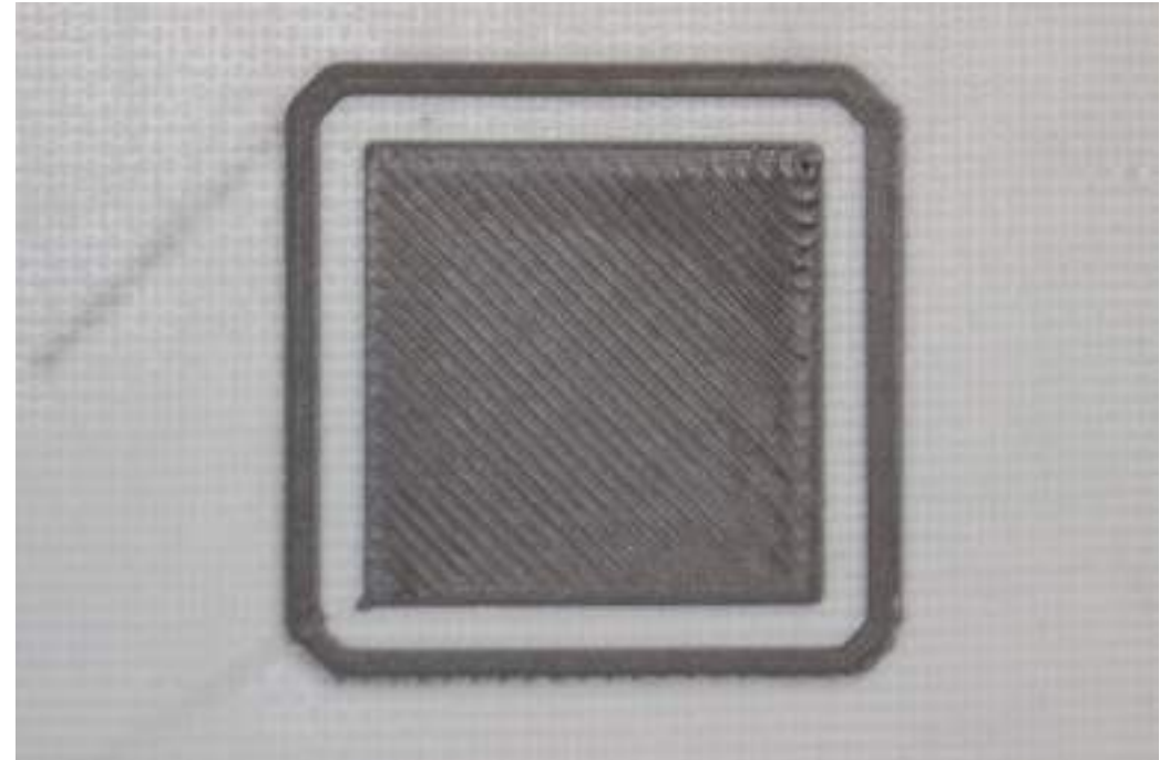
Correctly printed first layer
