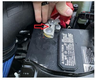
6. Install the intake assembly on the truck, push the intake mounting stud into the factory grommet, push the silicone coupler on to the lower intake manifold, take care positioning the intake tube making sure there is adequate clearance at the maf and battery cable positions as shown.
