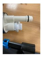
2. Push the billet body onto the O ring. You will have to work your way around the pump outlet with a pick or plastic thin tool to gently tuck the o ring into the coupler. After the O-ring is started, push the body down until it stops.install the C retainers with the provided bolts.
