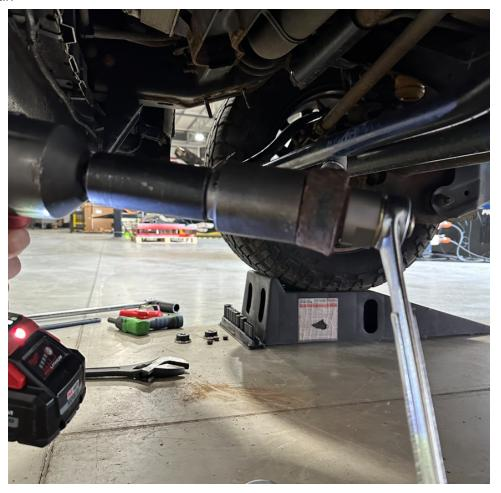
5. After removing the bushing from the trac bar it is critical that the faces be cleaned off as shown. We recommend using an abrasive pad or sandpaper. The new bushing will utilize the faces of the bar.
