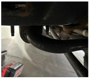
2. Drop the sway bar down. This will allow access to the main trac bar bolt and nut on the frame bracket. Remove the nut and bolt. We recommend loosening with a breaker bar and wrench and then removing the rest of the way with an impact.
