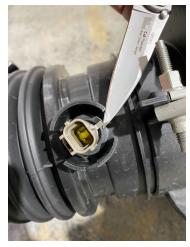
3. Remove the o-ring and install the IAT sensor into the SPE intake.
