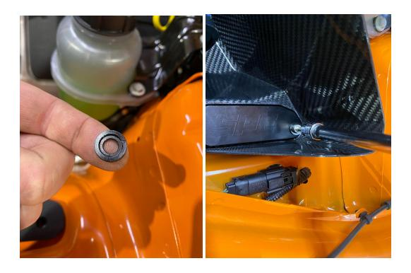
9. Push the coolant hose mount tie onto the stud.
