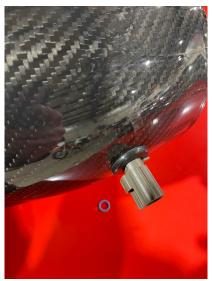
4. Install the Delrin isolator on the box mounting position.
