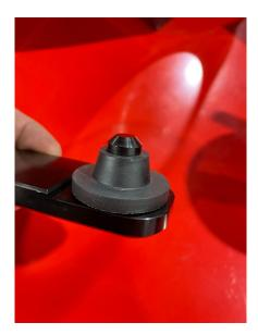
8. Install the mounting clamp into the box with the included allen bolt and washer. The washer is a wedge shape. Point the arrow towards the rear of the car. The box can be slid forward or backward in the mount. (This allows for adjustment due to irregularities in manufacturing of the vehicle.)
