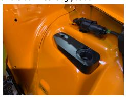
5. Prep the filter box/shield and install the included M6 bolt and nut as shown. This is for the coolant hose stud mount tie. Set the box into position and look at where the hose retainer locates. Mark its location. You will need to drill a 1/4" hole, then install the stud and nut.
