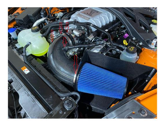
\*\*\*\*\*\*Make sure to clean and oil the filter as needed. Any standard filter cleaning kit and oil will be sufficient.
