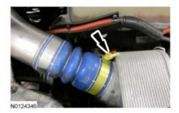
**1.** Loosen the clamp and disconnect the Charge Air Cooler (CAC) inlet tube from the CAC and position aside by twisting.
