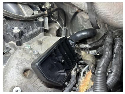
**10.** Clean the valve cover and install your SPE Recirculating CCV lower body with the provided o-ring and M6 bolt. Install the rear 2 bolt <sup>3</sup>/<sub>4</sub> hose venturi adapter flange to the rearmost hole on the valve cover with the provided bolts make sure to install the provided o-ring. Install the P-trap style hose. Use the provided zip ties on the hose to clamp the hose to the barbs.
