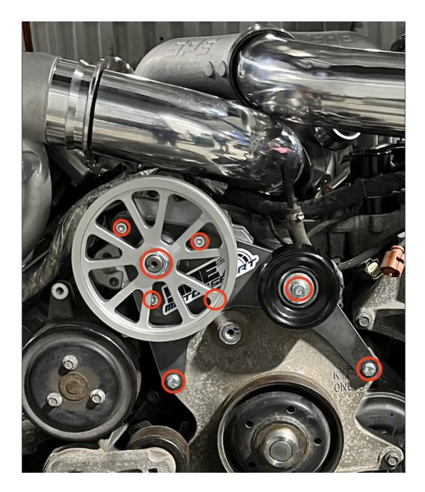
6. Install the (3) supplied M8x1.25x150mm bolts into the pump bracket and tighten evenly while supporting weight of pump to ensure no binding occurs. Torque bolts to 20 ft-lbs. Using the supplied washer and nut, install the supplied CP3 pulley. Torque to 75 ft-lbs. Install the lower portion of the high pressure fuel line onto the previously installed fuel rail feed fitting. Torque the upper and lower high pressure fuel line nuts to 40 ft-lbs.
