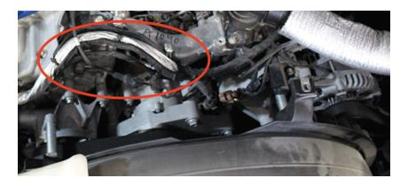
2. Cut zip ties and remove the two plastic wiring harness guides at the top side of the engine behind the front accessory drive.
