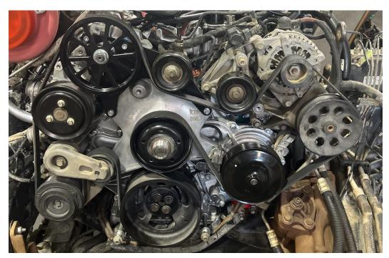
8. Install the serpentine belt as shown. Re-install the factory cooling fan. The fan shroud/stator mount that attaches to the secondary water pump will need to be removed all together it will no longer be needed. The shroud can be trimmed to give it a cleaner look.
