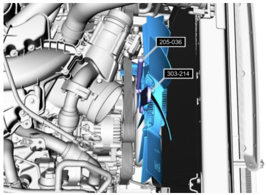
4. Unplug cooling fan speed sensor harness. Loosen and remove bolt holding cooling fan wire harness assembly. Remove the factory serpentine belt and both upper idler pulleys. Loosen cooling fan hub nut. Remove the fan shroud support stud on the secondary water pump.
