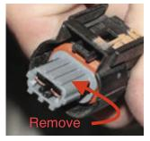
3. Locate and unplug the factory CP4 wire harness connector. Re-route the harness toward the front of the engine, exposing the connector for easy access. Remove the gray locking sleeve from the connector. Pull outward to remove it. Then plug the male factory CP4 harness into the female
