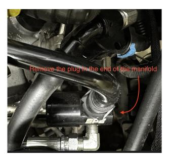
12. Remove the ¼ inch plug in the end of the fuel manifold on the CP4 fuel supply tube. Install the 90 degree supplied fitting. Install the -6an 90 hose end and route the hose to a 90 degree hose end on the CP3 Feed fitting. Take care in routing the hoses away from heat and sharp objects. Before final tightening, make sure the hoses are free of debris.
