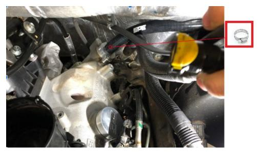
10. Clean the valve cover and install your SPE CCV flanges, matching the round block off to the most forward valve cover prevision and the venturi fitting to the rear most hole in the valve cover (use supplied hardware). Install the silicone hose and clamp, routing the hose over top of the brake booster.
