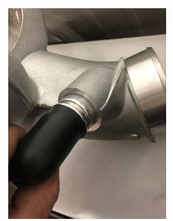
11. Install the rubber cap on the lower intake manifold pushing all the way down, use the supplied zip tie to secure it in the groove of the fitting.
