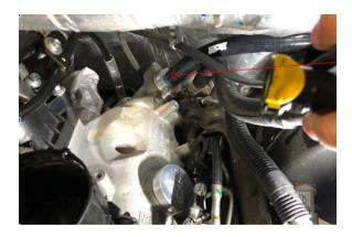
2. Install the Internal catch can below the 2 bolt flange. Install the O ring and use the supplied longer hardware. Push the ICC towards the front of the vehicle and tighten the bolts.
