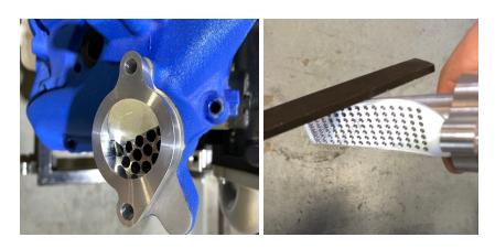
**Note**. It may be necessary to file or sand the edges to get the baffle to drop all the way in. This is due to casting irregularities from Ford. It's usually not necessary to remove much material if any. Try to remove an even amount from both sides with a file or angle grinder. You can normally see where the rubbing is occurring. Remember to take small amounts off at a time.
