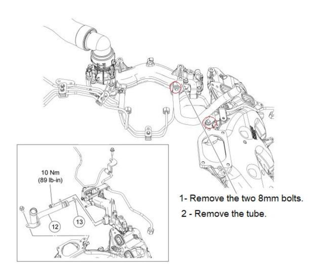
3- After removing the tube and disconnecting the heater hose, you will now need to trim the tube. Below is the simplest way to measure: cut the pipe with a standard tubing cutter.
