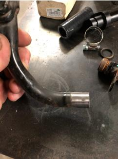
5- Assemble the o-ring onto the fitting, lubricate the o-ring, and install the fitting with the included hardware (tighten to 89 lb-in)
