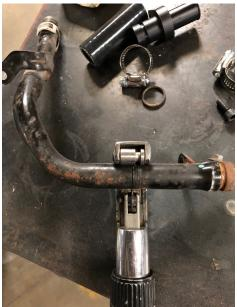
4 - Once the tube is cut, deburr, and clean the end.
