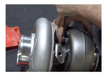
7. Install the large 2 x 28 o-ring into the turbo drain flange. Mount the flange to the turbo using the two included 3/8x16x3/4 Allen bolts.
