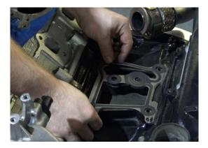
3. Install the pedestal plate with M10x1.5x30 bolts, M10 washers. Torque to 35ftlb.
