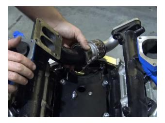
6. Using a 13mm wrench, loosen the turbo compressor and turbine housing bolts so they can be clocked correctly for fitment.
