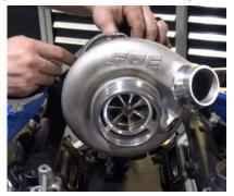
15. Using the supplied plug or cap, block off the turbo coolant feed from the cross over.
