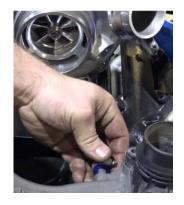
16. Install the lower intake manifold with supplied adapter and scroll clamps. The SPE on the adapter will clock to about 1 as pictured. Then install the upper intake manifold.
