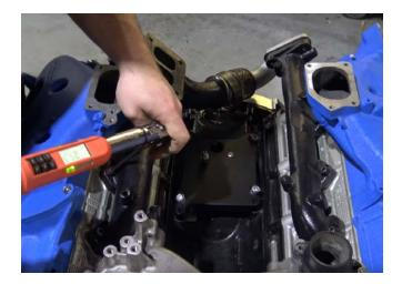
5. Using an 11mm or 7/16 socket, install the factory up pipe clamp and tighten.
