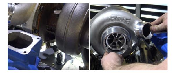
Once everything is clocked correctly you can proceed to tighten the bolts and clamps. Using an 8mm ball allen socket, install the T4 flange gasket with the included four M10x1.5x25 (12.9 black) Allen bolts.
