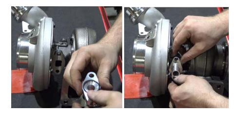
8. Next take the oil drain tube and cut ½ to 5% of an inch off of each end so the tube fits properly. The amount necessary to cut will vary depending on the turbo frame size.
