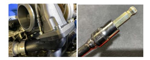
13. Install the downpipe upper elbow with the included s300 to 2015+ downpipe adapter. Use the included V-band clamp and a 2015+ factory clamp. 20+ trucks will require you to cut the tab on the factory downpipe. \*\*NOTE SPE Recommends the MBRP FAL460 downpipe (or similar) for all year trucks.
