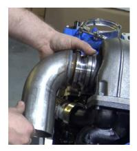
14. Install the supplied ¼ NPT x -4 AN oil feed fitting into the top of the turbo with thread sealer. Proceed to install the premade hose (no sealer) from the pedestal to the top of the turbo, keeping it away from the exhaust housing.
