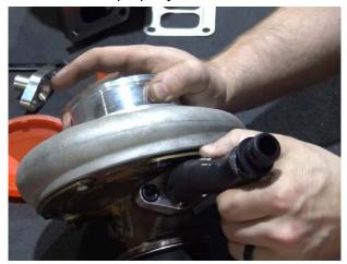
11. Dry fit the turbo and get the drain clocked properly along with the housings before tightening anything. The oil inlet at the top of the turbo center section should be flat. The SPE logo on the compressor cover should clock down slightly.
