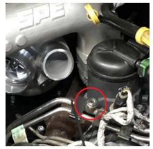
18. On the hotside factory intercooler pipe, you will need to cut the metal band off for the coupler on the intercooler side of the pipe. This is so you can remove the factory coupler and replace it with the SPE provided 3" coupler as shown. Attach the hotside pipe as shown clip on the turbo side coupler first. Then, tighten the intercooler side coupler with the provided T bolts.
