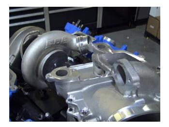
17. On the 11-14 ONLY install the provided to fuel temp sensor plug as shown reusing the copper washer off of the sensor on the plug. Most tuning companies will be utilizing the harness side already for a switch.
