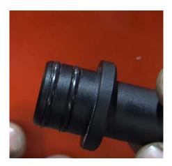
10. Assemble the turbo drain pieces as pictured. Slide on the two provided #10 clamps leaving them loose until clocked properly.
