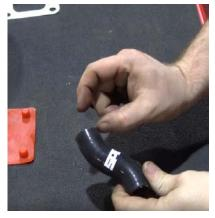
9. Next install the two 2x18 o-rings onto the pedestal drain fitting and lube them thoroughly.
