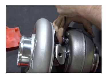
7. Install the large 2 x 28 o-ring into the turbo drain flange. Mount the flange to the turbo using the two included 3/8x16x3/4 Allen bolts.
