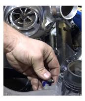
16. Install the lower intake manifold with supplied adapter and scroll clamps. The SPE on the adapter will clock to about 1 as pictured. Then install the upper intake manifold.
