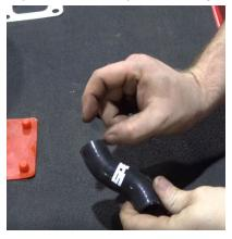
9. Next install the two 2x18 o-rings onto the pedestal drain fitting and lube them thoroughly.
