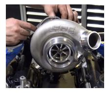
15. Using the supplied plug or cap, block off the turbo coolant feed from the cross over.
