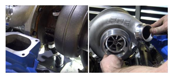
12. Once everything is clocked correctly you can proceed to tighten the bolts and clamps. Using an 8mm ball allen socket, install the T4 flange gasket with the included four M10x1.5x25 (12.9 black) Allen bolts.
