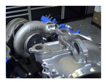
17. On the 11-14 ONLY install the provided to fuel temp sensor plug as shown reusing the copper washer off of the sensor on the plug. Most tuning companies will be utilizing the harness side already for a switch.
