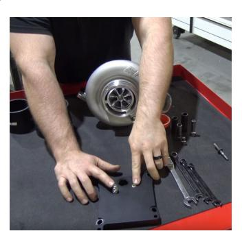
2. Install the gasket for the pedestal on the block.
