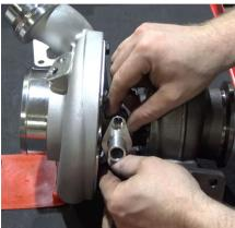
8. Next take the oil drain tube and cut ½ to 5% of an inch off of each end so the tube fits properly. The amount necessary to cut will vary depending on the turbo frame size.
