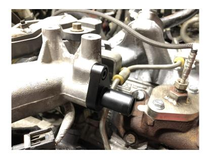
4. Install the supplied silicone hose and #10 clamp loosely on the fitting as shown.
