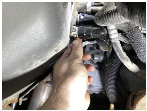
6. Remove the white retaining clip left behind by the factory quick connect.
