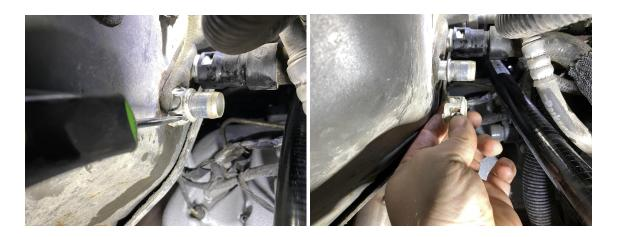
7. Install the supplied 90 degree quick connect adapter as shown. Trim the hose to fit install on adapter with the supplied #12 clamp. Tighten clamps.
