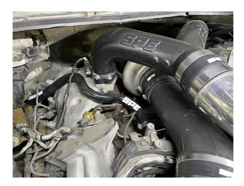
5. Remove the heater hose rubber tube. Disconnect the quick disconnect end from the heater core. Push in on the elbow fitting and squeeze the white tabs then pull back on the fitting. **Note:** This may be easier with the inner fender removed.
