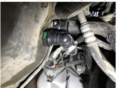
8. Remove the radiator degas hose T assembly. Install the included hose, then route and tighten clamps as shown below.
