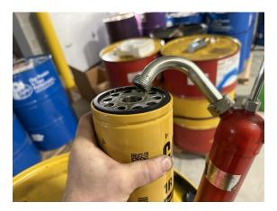
7. After installing the filter and topping off your oil, start the vehicle then recheck your oil levels, also being sure to check for any leaks.
