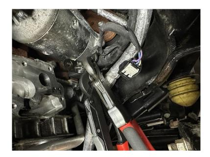
4. Transfer the temperature and pressure sensors into the new housing. The 11-19 trucks have taper threaded NPT sensors so be sure to use thread sealant. The 2020+ engines have oil pressure/temperature sensors built into one unit. This sensor is o-ringed so it doesnt need sealant. At this time you can install the provided plugs in the auxiliary oil ports and/or set them up for your intended use.
