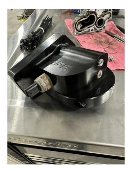
5. Install the new provided gasket into the housing. Then, install the housing with the provided stainless 5mm drive allen bolts. Torque to 100 IN-LB. Connect the sensors.
