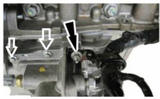
3. Due to the size of the SPE housing the wire holder/clamp will not be reused. Using pliers, remove it from your harness. Some trucks may vary in the style holder.
