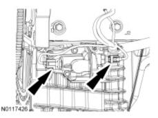
2. Remove the 10mm nut for the wiring harness. Then remove the rest of the 8mm bolts.
